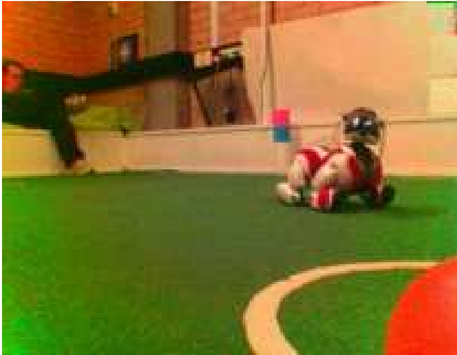
Figure 1.2: The same arrangement as in Figure 1.1 , this time taken with the camera of another robot. Note the low resolution, the pixel noise and the vignetting near the corners of the picture.
